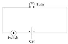
A diagram which shows how different components in a circuit have been connected using conventional symbols for the components is called a circuit diagram.
